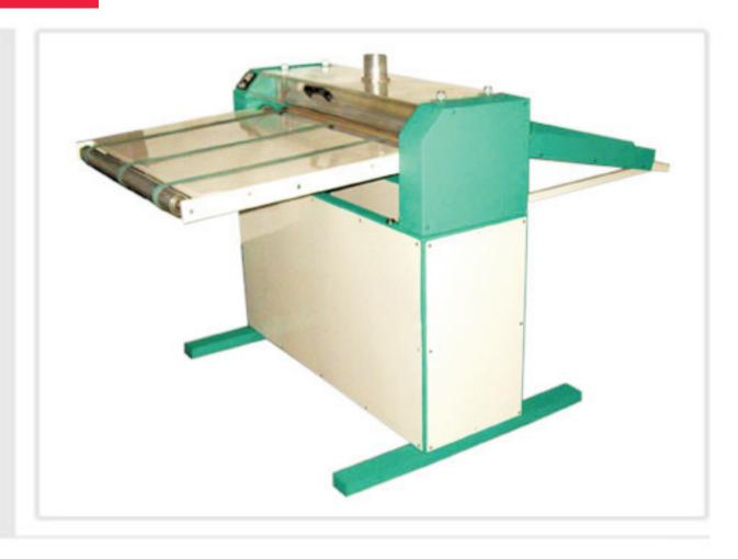
Some substrates are corona-treated when they are manufactured. Many of these substrates require a surface energy boost to match a particular ink or coating. This is done with **corona pretreaters** on the press just prior to the Printing / coating application point.
