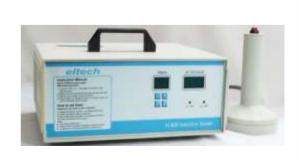
Induction sealing is a non-contact heating process, which is used to bond a foil disk or to seal the opening of a container. The technique provides the user with a tamper evident seal.
